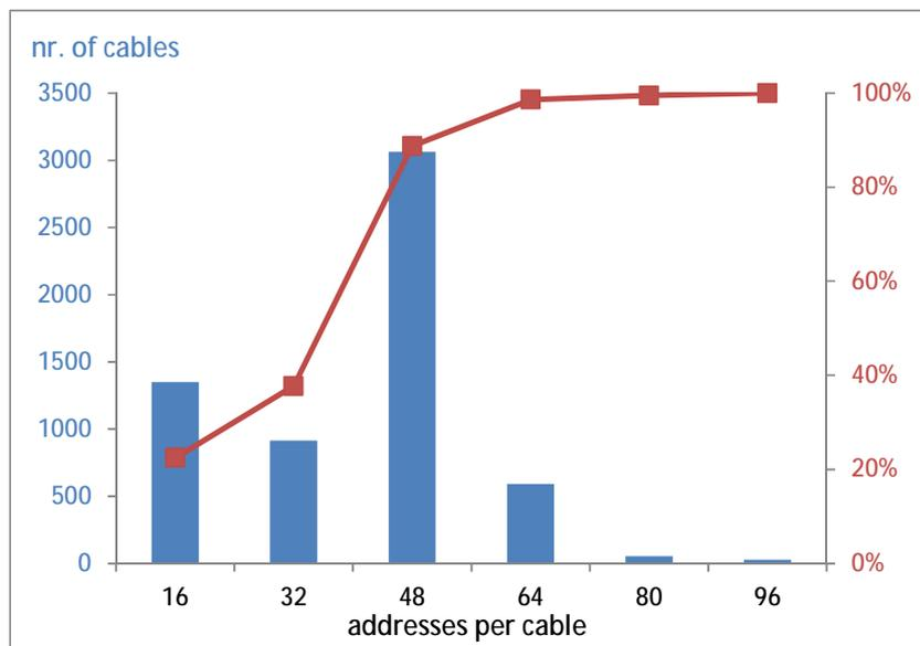
**Figure 2: Distribution of the number of unique addresses connected on the 100'' cables in which all connected addresses are located within 200 m (EC-length).**
