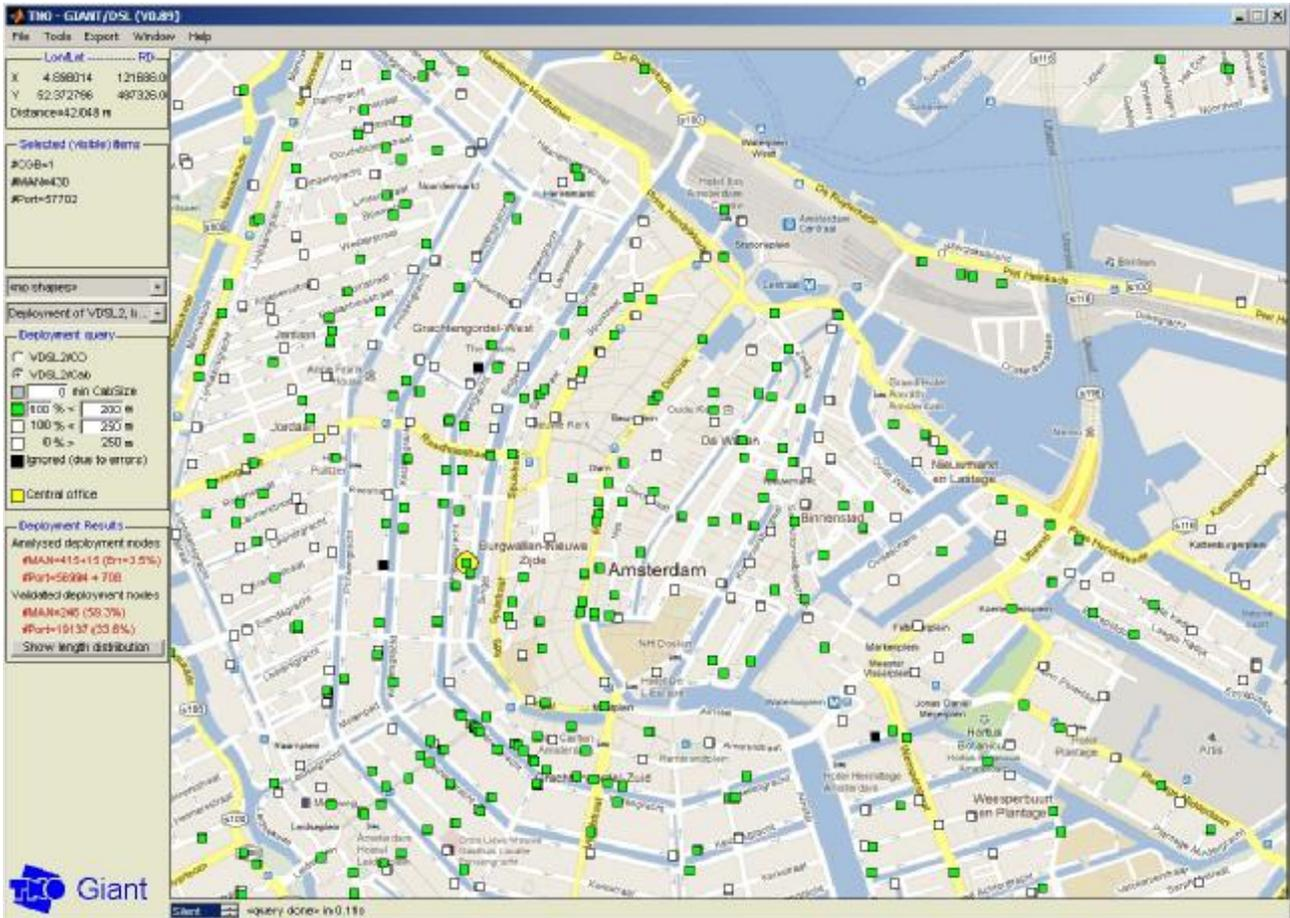
**Figure 3: All Street cabinet locations in central Amsterdam. This figure illustrates the large deployment opportunity (green colored cabinets) for G.fast in this area. The detailed numbers shown in the figure may differ from the numbers in the text due to e.g. a different selection of cabinets, and a cabinet-centered approach instead of a cable-centered approach**
