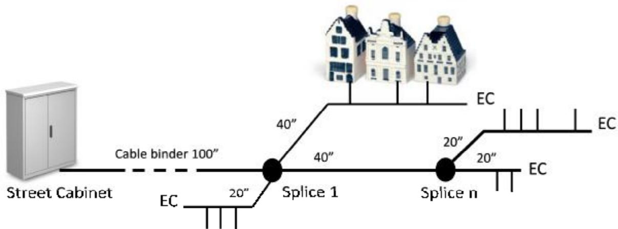
**Figure 1: Schematic example of a typical (secondary) access network in Amsterdam.**
