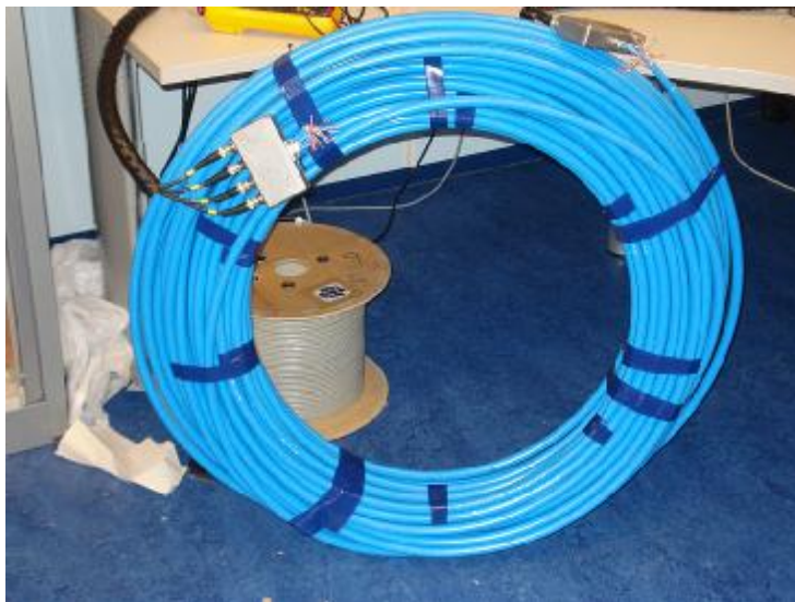
Figure 1: The 6x4x0.5 KPN Access cable for which the transfer characteristics were measured.
