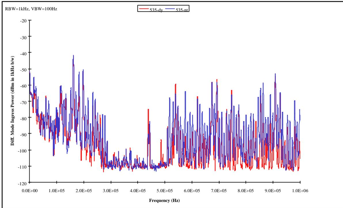
Figure 1. Measurements on ingress noise, presented by BT in Monterey (TD26, dec 2000, file 004t26.pdf), representing "differential mode ingress levels on rural overhead line L535"
