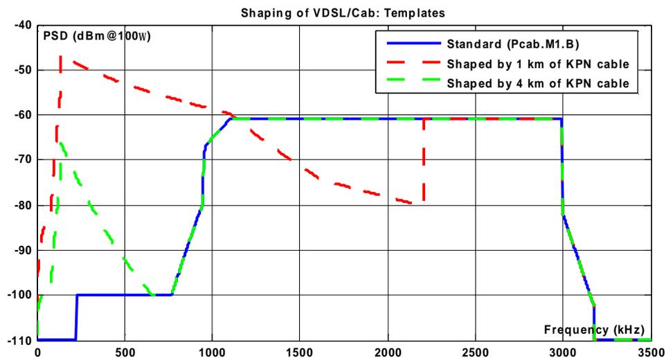
Figure 2: Length dependency of PSD shaping of VDSL2/Cab. Examples for ‘near’ cabinets (1 km) and ‘far’ cabinets (4 km)
