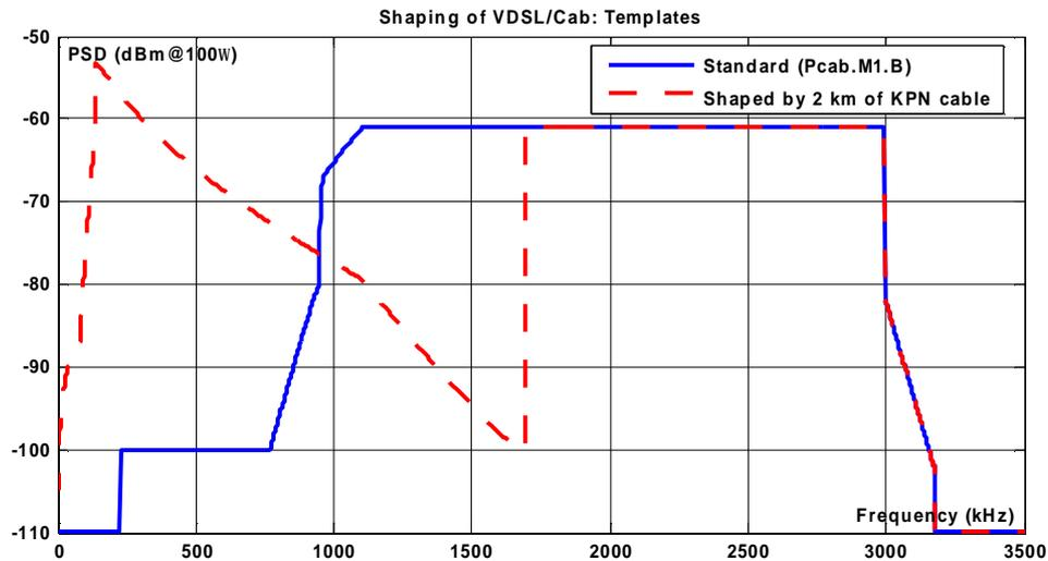
Figure 1: Generic concept of PSD shaping of VDSL2/Cab over the full band between 0 to 2.2MHz
