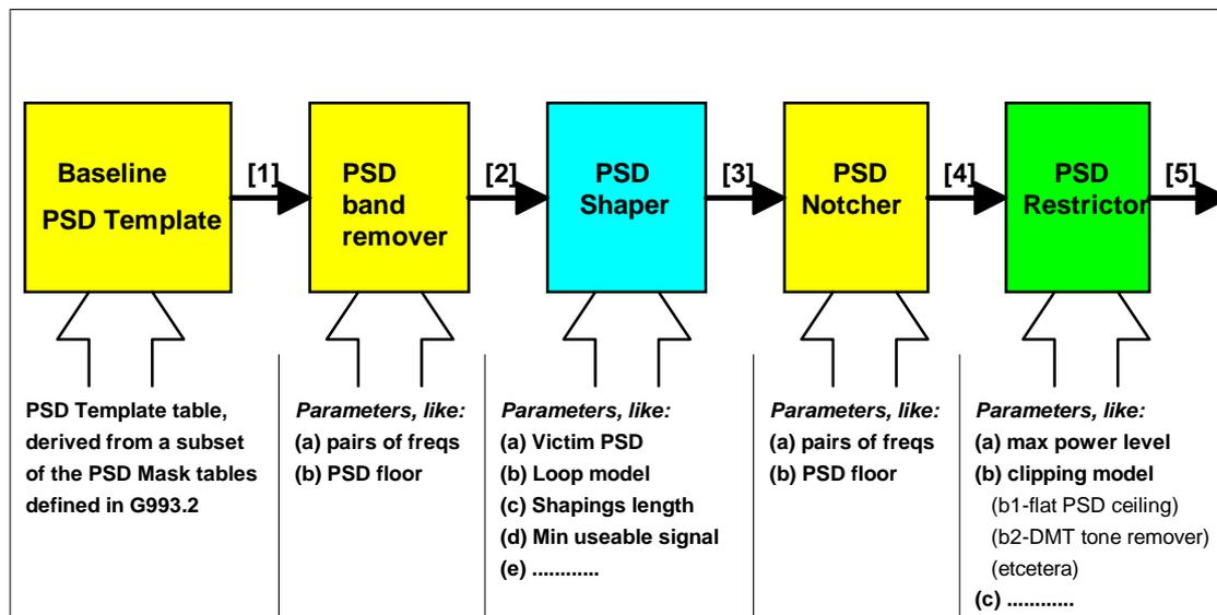
*Figure 1: Building blocks of a VDSL2 transmitter model, to define a wide range of PSD templates with only a few PSD tables and formulas.*
