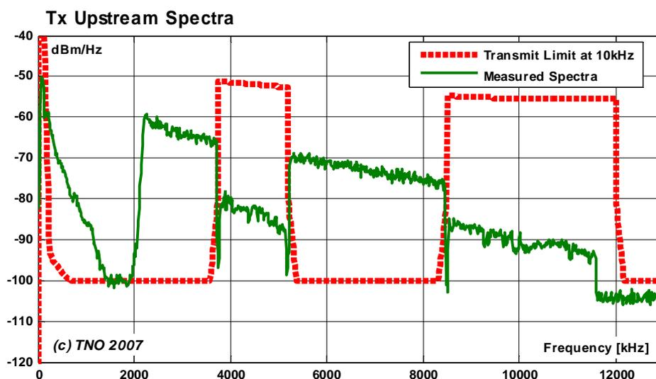
Figure 2. Spectrum measured at the NT side of the loop (at CP) when the modem applies the preferred amount of upstream power back-off.
