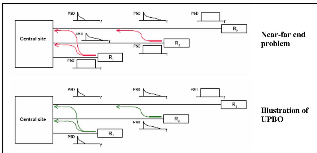
**Figure 1. When CP-modems are distributed, and all upstream transmitters transmit at equal power, then the long loops are in a disadvantage.**
