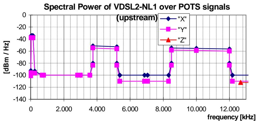
Figure 4: Spectral Power for "VDSL2-NL1" upstream *transmit* signals, as specified in table 1.
