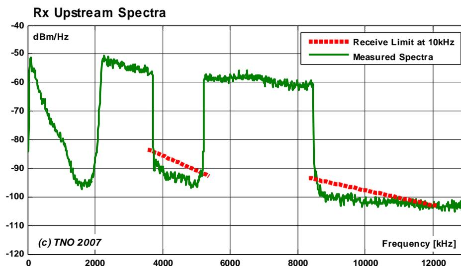
Figure 3. Spectrum measured at the LT side of the loop (at Cabinet) when the modem applies the preferred amount of upstream power back-off.
