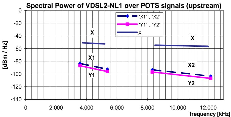
Figure 5: Spectral Power for "VDSL2-NL1" upstream *receive* signals,
