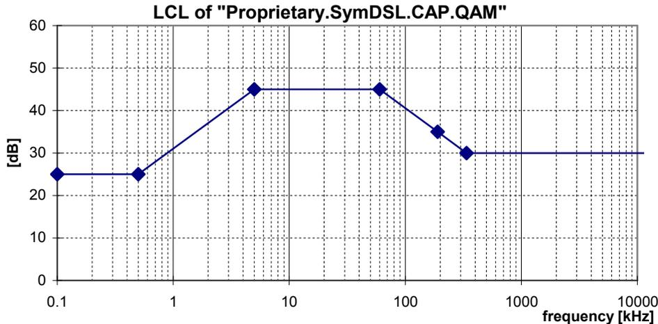
Figure 11: Minimum LCL for a "Proprietary.SymDSL.CAP.QAM" signal source
