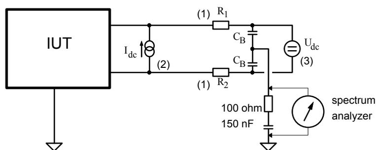
**Figure 47: Measurement method for longitudinal output voltage (LOV)**
