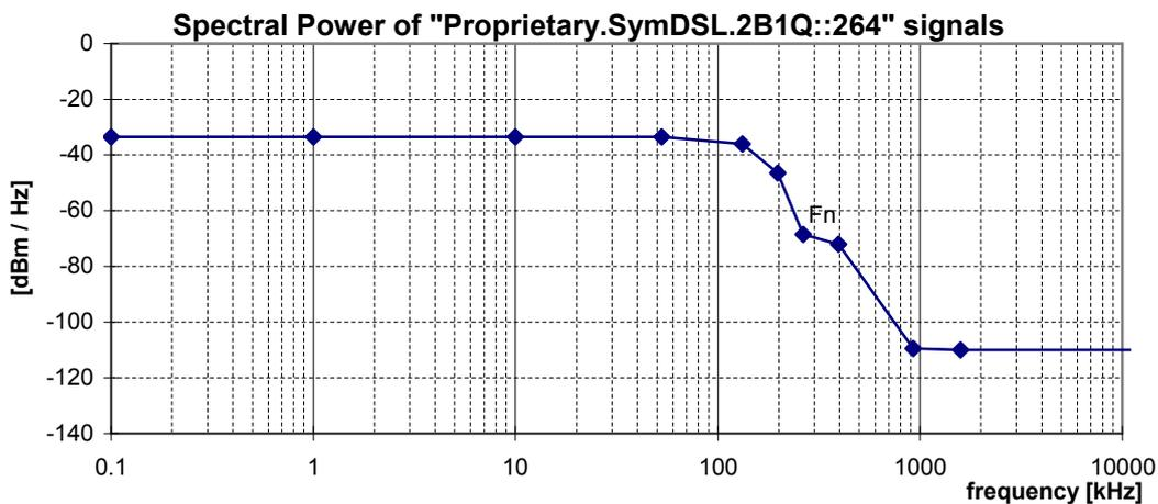
NOTE: These curves are dependent on the Principal frequency  $F_N$ , and that this figure shows an example only.
