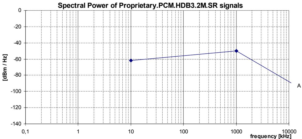
Figure 36: Spectral Power, for Proprietary.PCM.HDB3.2M.SR signals, as specified in table 60
