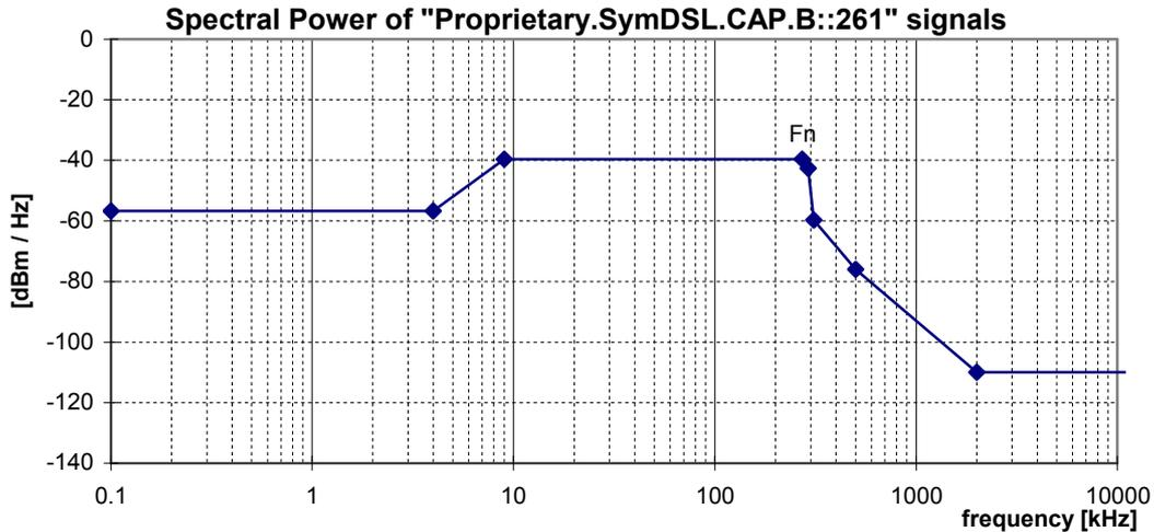
NOTE: These curves are dependent on the Principal frequency  $F_N$ , and that this figure shows an example only.
