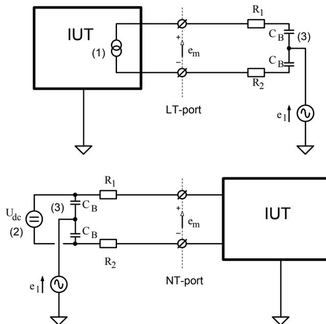
**Figure 48: Measurement method for longitudinal conversion loss**
