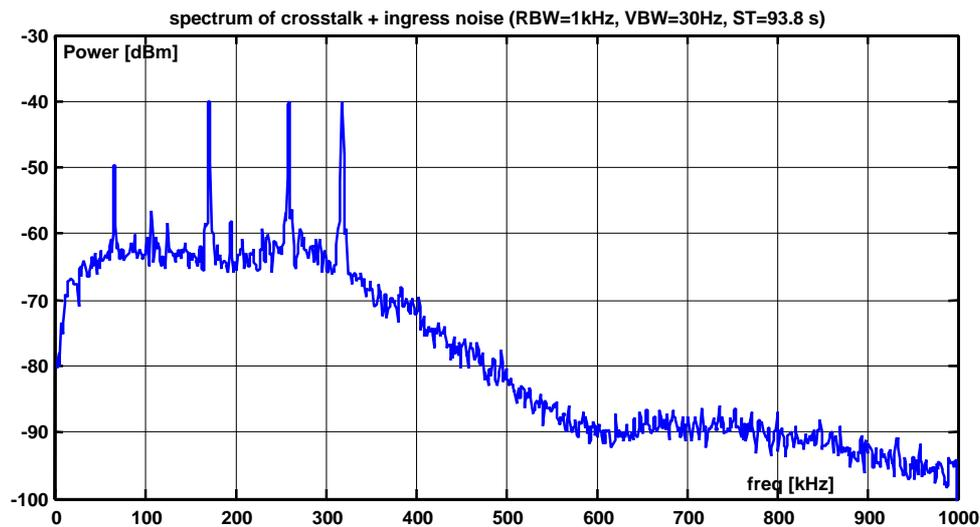
**Figure 3.** Example spectrum of the combination of crosstalk and ingress noise
