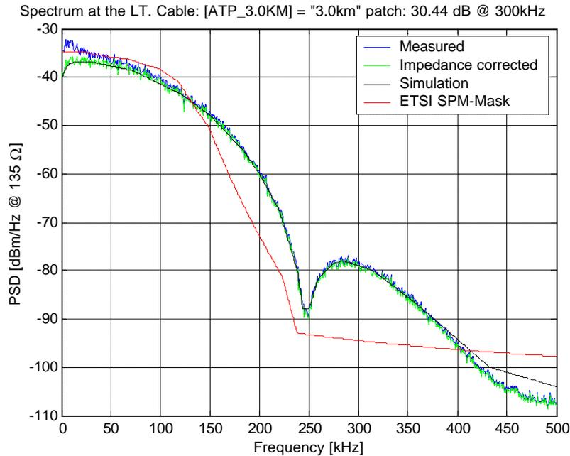
Figure 1. Measured PSD of the prototype SDSL look alike modem under test, as it can be observed at the LT-side of the line.
