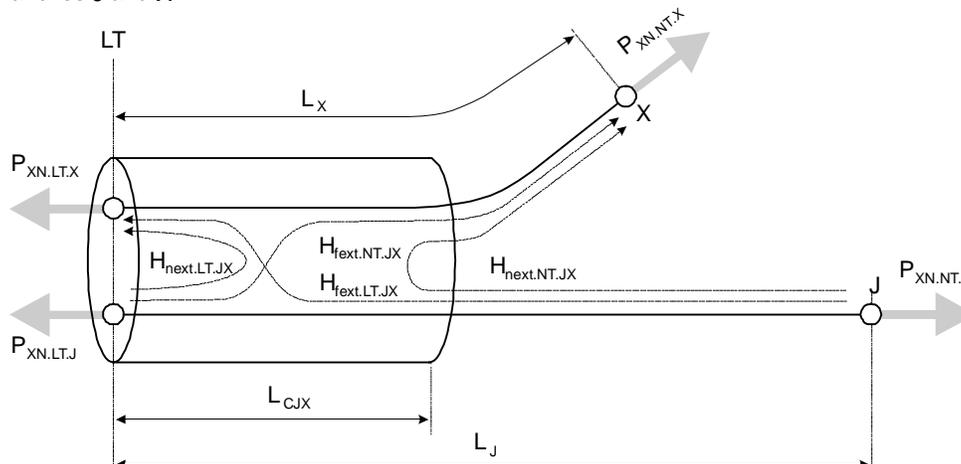
**Fig. 4 Transmission parameters of cable tree branches  $J$  and  $X$**
