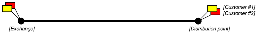
Figure 1: Example of a two-node cable section topology
