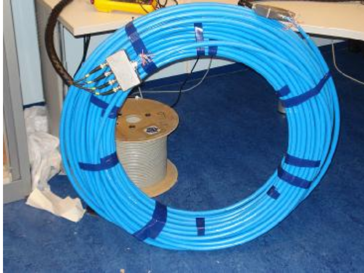
Figure 1: The 6x4x0.5 KPN Access cable that was used in the measurements. This cable corresponds to the “T05u” cable model described in the Appendix I of the draft G.fast standard.
