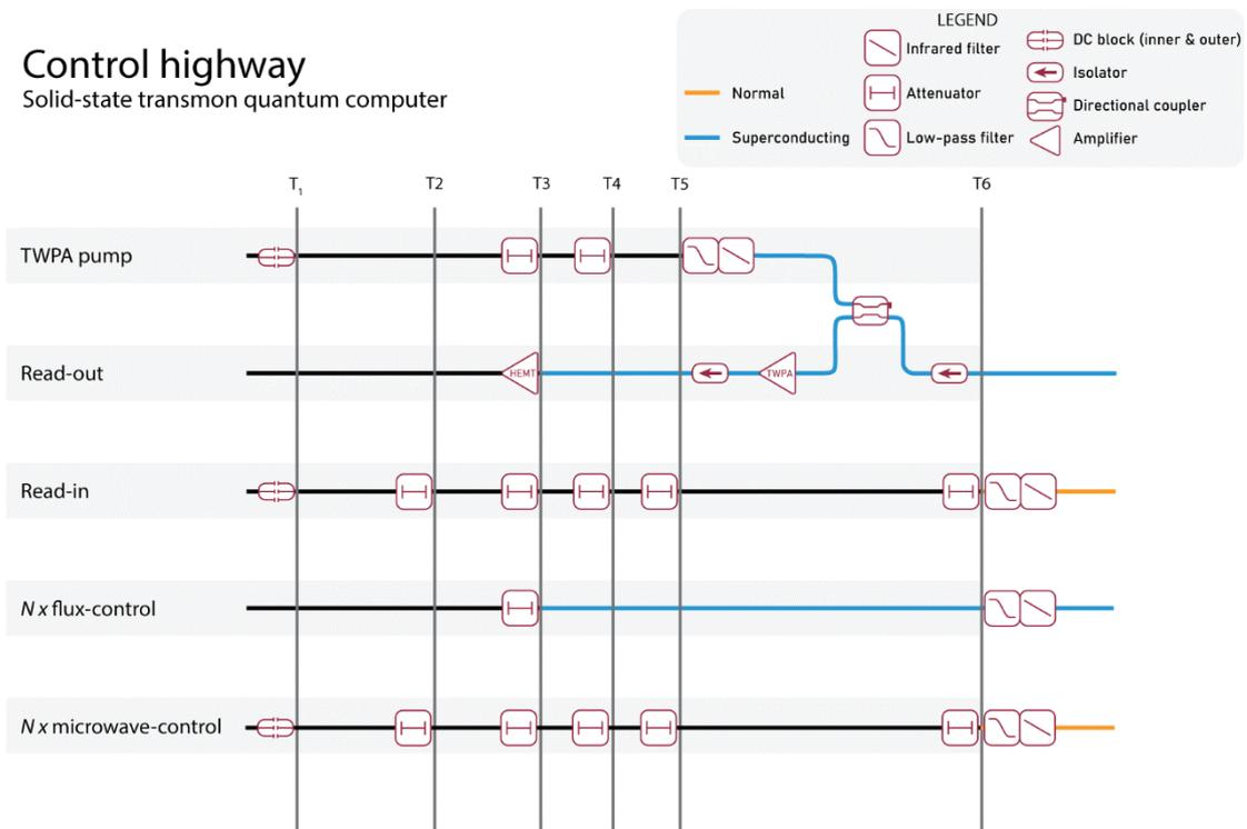
**Figure [E.6.1] An example of a control highway applicable to a particular transmon architecture.**
