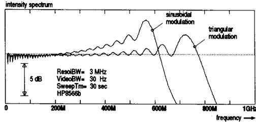
Fig. 3. Measured output spectrum of the synthetic noise source with 10 MHz modulation, 17 MHz linewidth laser, approximately 10 m differential delay and 0.8% bias current modulation.
