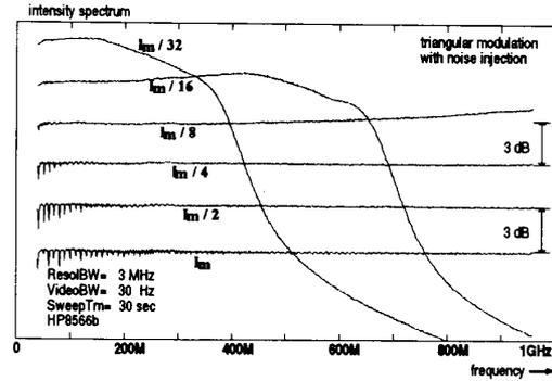
Fig. 6. Measured synthetic noise spectrum for various modulation depths, related to an arbitrary maximum modulation current  $I_m$ . (approximately 12% of 60 mA bias current).
