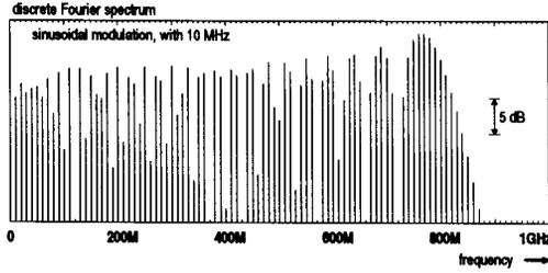
Fig. 2. The photo current has essentially an FM line spectrum, with equidistant lines.
