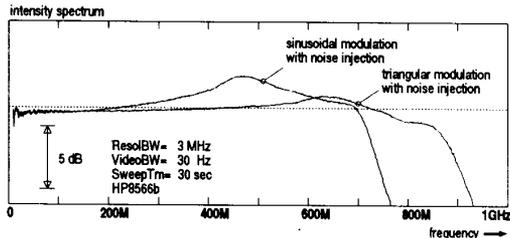
Fig. 5. Measured output spectrum of the synthetic noise source with noise injection. The periodical and random modulation currents were approximately 0.8% and 7% of the laser bias current (60 mA). Increasing the spectral peak offfigure 4 to  $f = 1/(2 \cdot \tau)$  will relax the injection level requirements.
