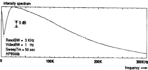
Fig. 4. Measured spectrum of the (pink) noise that was injected to broaden the individual comb-lines.
