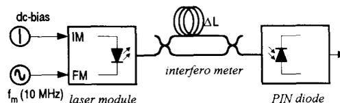
Fig. 1. Basic setup of a synthetic noise generator.  $\Delta L = 10$  m, 1530 nm DFB laser, 60 dB isolation.
