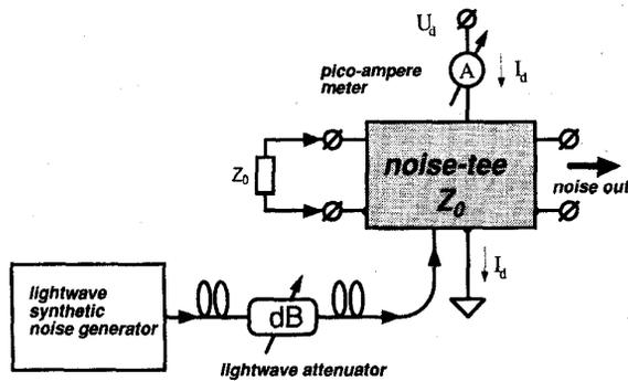
Fig. 2. Matched noise-tee configuration as an implementation of an electrical noise source with variable output level. The ratio between photo current  $I_d$  and spectral current density ( $\sqrt{S_{ic}}$ ) of the excess-noise is insensitive to optical power variations.
