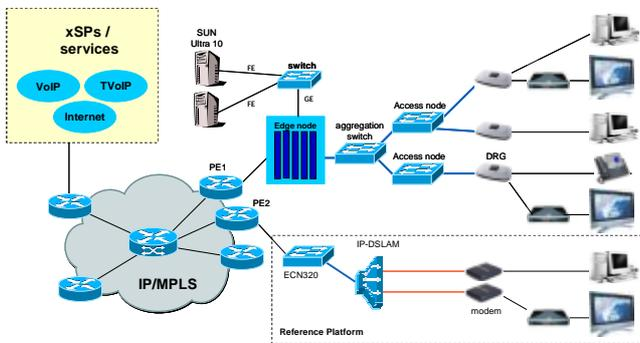
Figure 1: Detailed overview of the MUSE lab trial test and evaluation set-up
