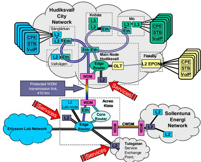
Figure 2: Schematic illustration of the testbed
