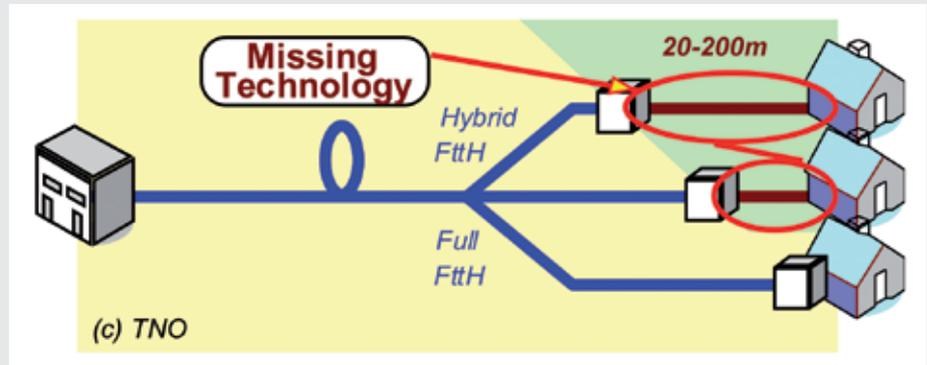
Figure 1: Hybrid copper fibre solutions to achieve Gb/s rates.
