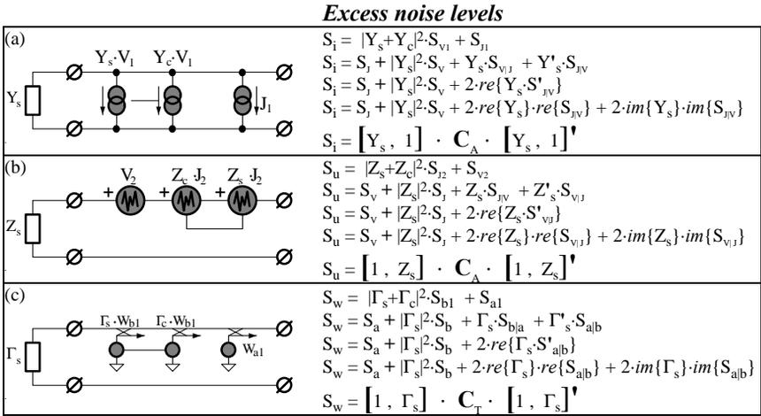
**Fig 7.8** Various related expressions for evaluating the device excess noise at specified source impedance. This excess noise equals the total equivalent input noise when the source impedances is cooled down to  $T=0$  Kelvin.
