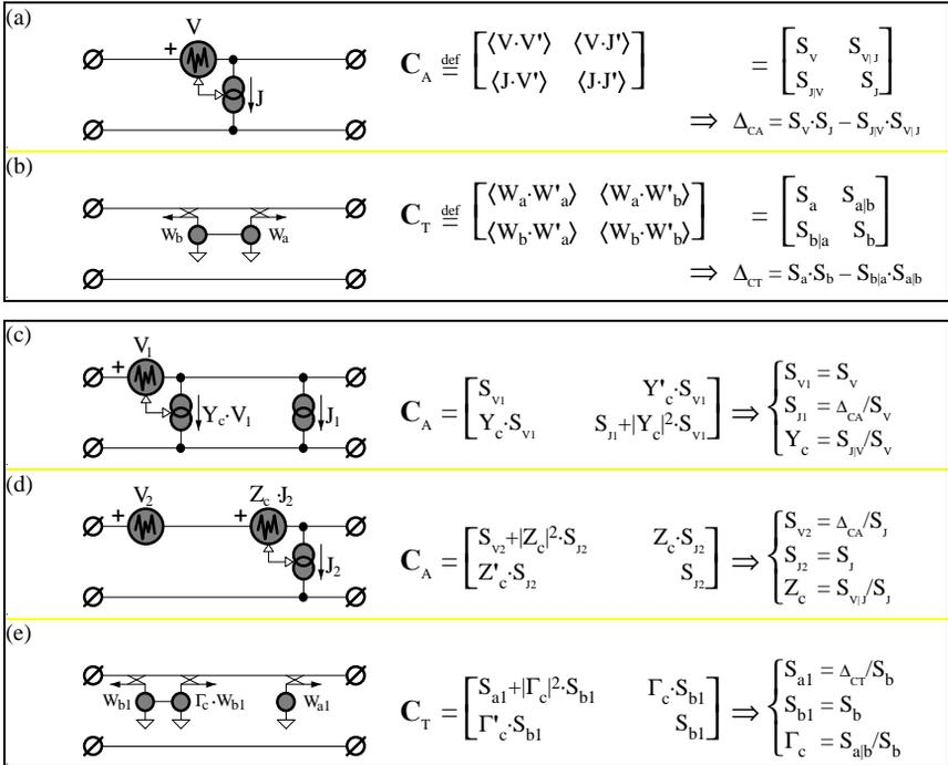
**Fig 7.7** Two (partly) correlated noise sources can be represented by two fully correlated sources and an additional uncorrelated noise source. This approach simplifies manual circuit analyses of input noise.
