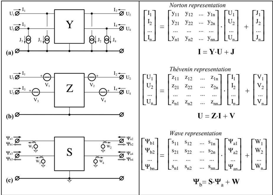
**Fig 7.3** Three basic blackbox models of multi-port networks comprising arbitrary (deterministic) signal sources. They are a generalization of the Norton, Thévenin and wave representations of one-port sources, as described in section 2.1.3. The exchangeable source power is [715]:
