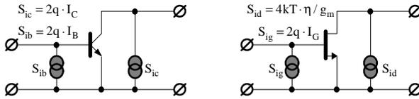
**Fig 7.12** Simple noise models for transistors. Most noise sources originate from shot noise associated with bias currents or leakage currents. The channel noise in the FET is represented acting as if the transconductance  $g_m$  is providing thermal noise. The correction factor  $\eta$  is a value close to one, to be extracted from measurements. The FET model ignores the influence of induces gate noise because its contribution is of minor importance when designing wideband amplifiers [406]
