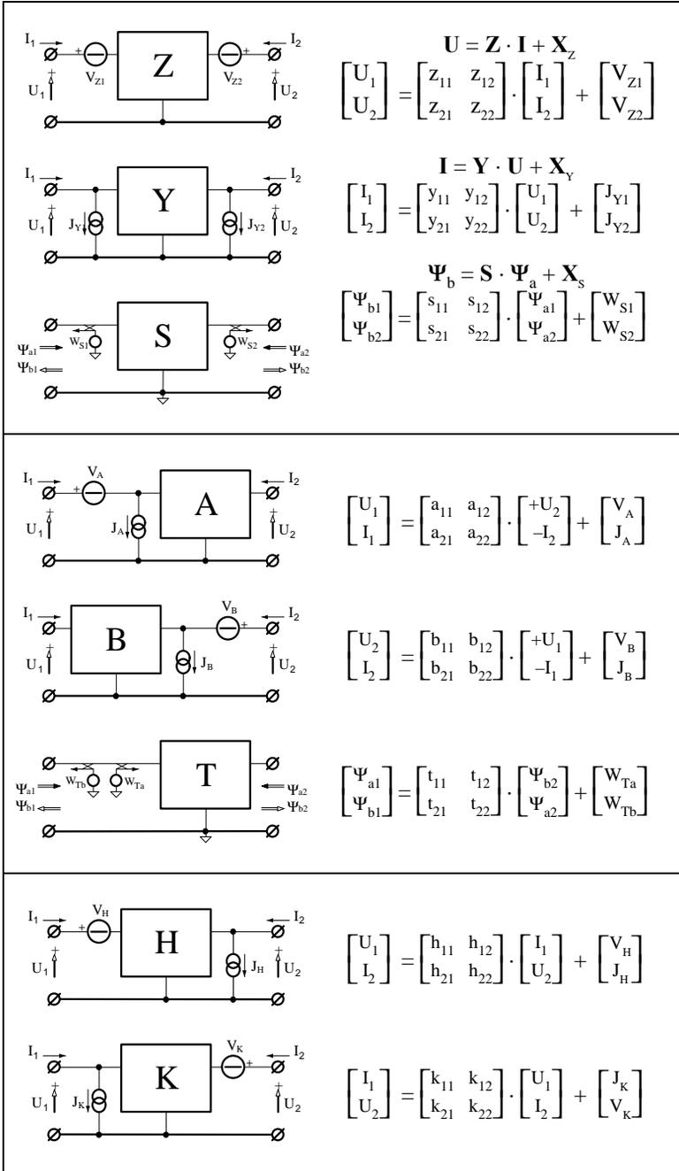
*Fig 7.5 Representations of internal (noise) sources of two-ports with two equivalent sources. The overall calculation effort is simplified when the associated matrix representation is used.*
