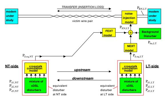
Figure 4: Flow diagram of the basic model for two-node topologies, for evaluating upstream performance
