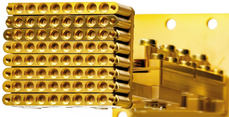
Figure 7.3. An example room-temperature node with 64 coaxial connections
